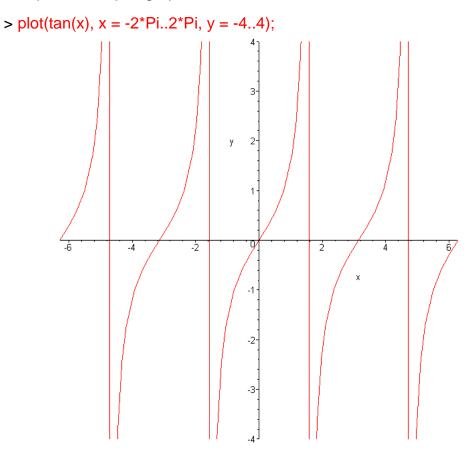
Parameter discont = true secures discontinuity of the plotted function graph on the chosen interval
