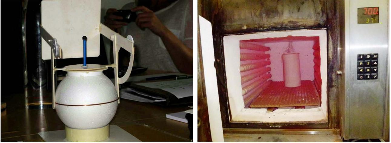
Fig. 1. A small model of thermal container (left photo). A cylindrical silicate specimen in the laboratory oven at the temperature 700 °C (right photo).
