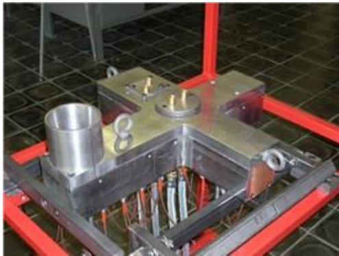
Fig. 3. Construction of casting die.
