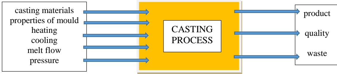
Fig. 5. Schematic entry-exit models casting system.
