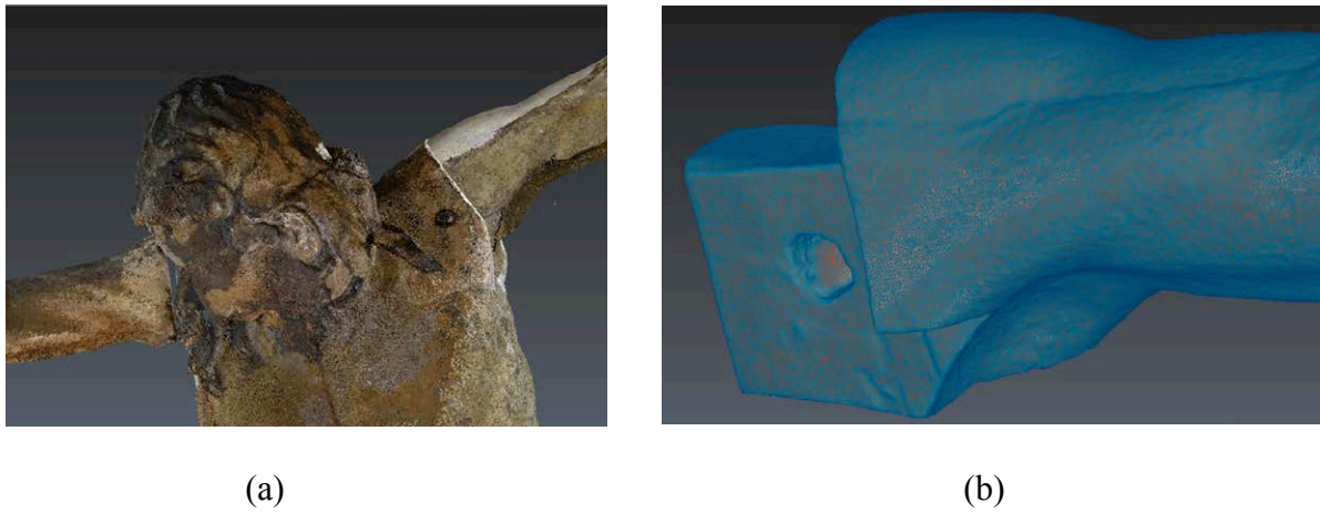
Fig. 4. (a) Photogrammetric survey during the restoration process: image of the 3D model with true colors mapped onto the surface. (b) Triangulated surface of the left arm joint.
